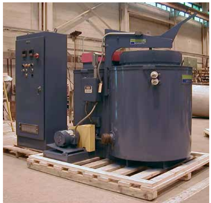
Figure 1 (A&B): Tempering furnace with cutaway view.
